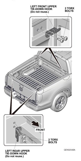
Install the left front bracket and left rear bracket to the left side bed lining with the four TORX bolts removed in step 1. Torque the TORX bolts to 20 N·m (15 lb·ft). Repeat on the other side. NOTE: Make sure that the brackets are installed in the correct position and orientation.
