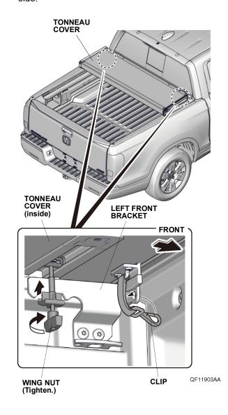
5. Open the tailgate, then unfold the tonneau cover.
