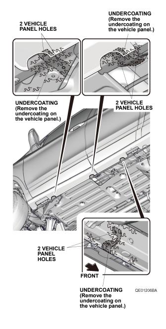
Loosely install the left bracket A, left bracket B, and left bracket C to the vehicle panel with six flange holts
