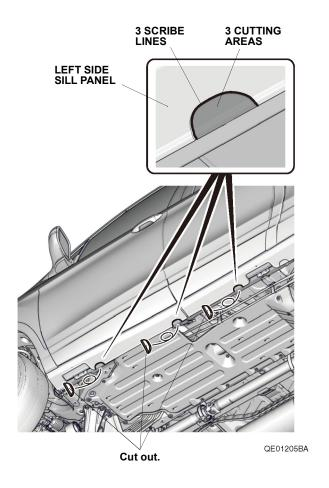
Remove the undercoating as shown. Apply touch-up paint where you removed the undercoating and allow it to dry thoroughly.
