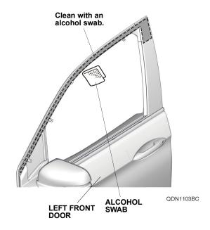
Attach a piece of masking tape to the end of the adhesive backings as shown. Peel back the adhesive backings partway and temporarily attach them to the front surface of the left front door visor.
