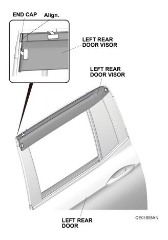
20. While applying light pressure against the left rear door visor, carefully remove the adhesive backings as shown. Make sure to push up on the brackets while removing the adhesive backings.
