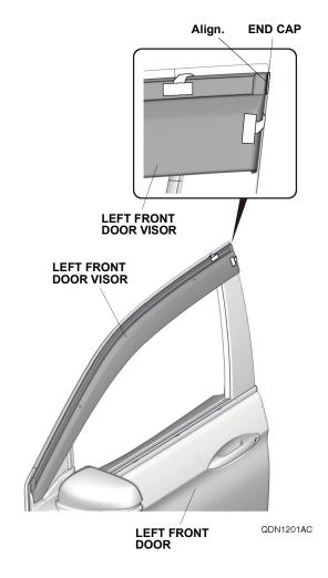
10. While applying light pressure against the left front door visor, carefully remove the adhesive backings in the order shown. Make sure to push up on the brackets while removing the adhesive backings.
