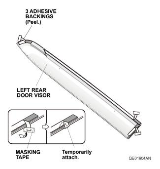
17. Adjust the two brackets A so the holes line up with the two holes on the left rear door visor.
