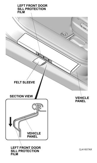
10. Starting from the center and working outward, use the felt sleeve to smooth out the left and right sides of the lower section on the left front door sill protection film. Move the felt sleeve in one direction only. If you see an air bubble, stop and gently peel up that section to work out the bubble. Work slowly, and keep pressure against the left front door sill protection film.
