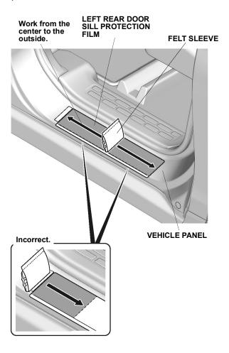
19. Starting from the center and working outward, use the felt sleeve to smooth out the left and right sides of the upper section on the left rear door sill protection film. Move the felt sleeve in one direction only. If you see an air bubble, stop and gently peel up that section to work out the bubble. Work slowly, and keep pressure against the left rear door sill protection film.
