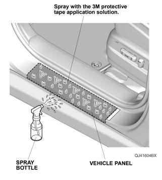
4. Remove the adhesive backings from the left front door sill protection film.
