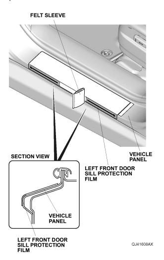
11. Using a shop towel, wipe off the 3M protective tape application solution. Allow the left front door sill protection film to dry thoroughly. Remove the masking tape.
