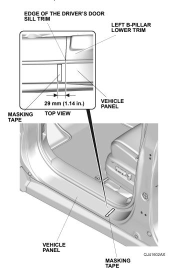
2. Using the alcohol wipe, thoroughly clean the vehicle panel where the left front door sill protection film will attach.
