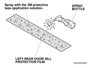
17. Line up the left rear door sill protection film with the curve end and masking tape as shown. Then, attach it to the vehicle panel.
