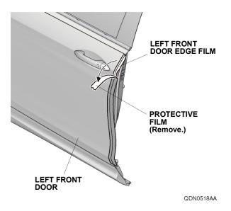
12. Starting from the center and working outward, use your fingers to fold the left front door edge film around the edge of the left front door. Move your fingers in one direction. Attach the left front door edge film over the seam sealant. Do not trim or damage the seam sealant.
