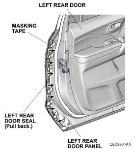
2. Using the alcohol swab, thoroughly clean the area where the left rear door edge film will attach.
