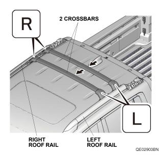
5. Line up the marks on the crossbars with the marks on the roof rails as shown. Tighten the eight thumbwheel screws to secure the crossbars to the roof rails.
