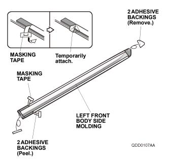
6. Line up the left front body side molding with the front and middle templates and attach it to the left front door as shown.
