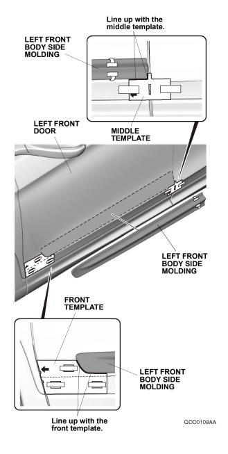
7. While applying light pressure to the left front body side molding, carefully remove the taped adhesive backings.
