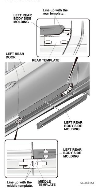
12. While applying light pressure to the left rear body side molding, carefully remove the taped adhesive backings.
