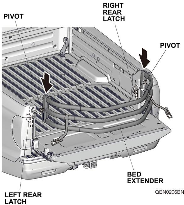
9. Carefully pull down the bed extender onto the tailgate.
