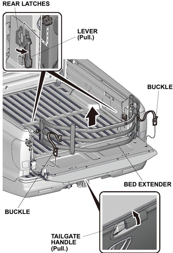
16. Insert the two pivots on the bed extender into the front latches. Push down on the bed extender until the parts are locked. Check that the bed extender is properly installed.
