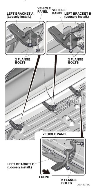
4. With the help of an assistant, install the left running board to the left bracket A, left bracket B, and left bracket C with six flange bolts. Torque the flange bolts to 27 N·m (20 lb·ft).
