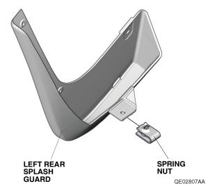
Install one spring nut on the left rear inner fender as shown.
