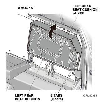
Secure the left rear seat cushion cover with the two fasteners.
