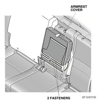
9. Pull down the armrest. Fit the left rear seat-back cover onto the left rear seat-back through the center seat belt. Insert the left seat-back cover under each head restraint guide.
