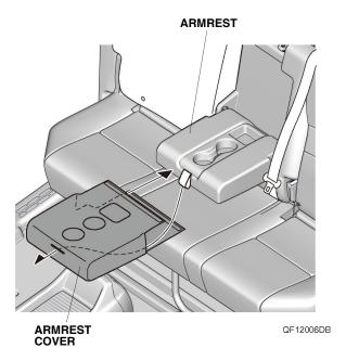
8. Raise the armrest. Pull out the armrest cover between the armrest and the rear seat-back and secure the armrest cover with the fasteners as shown.
