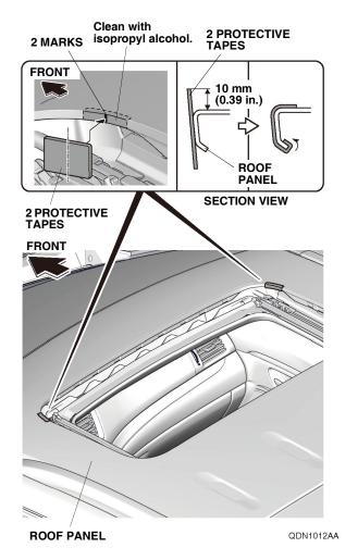
Remove the adhesive backing from the two
