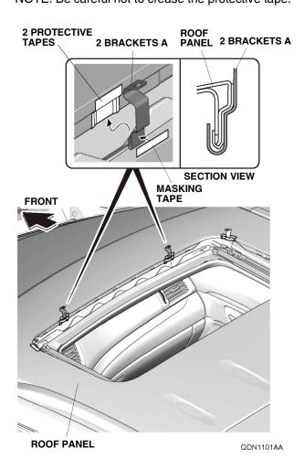
10. Set the moonroof visor on the vehicle roof in front of the moonroof opening, and adjust its position so the holes in the moonroof visor are lined up with the bracket A holes. Loosely install the moonroof visor to the brackets A with two screws and two nuts. Remove the strips of masking tape from the brackets A.
