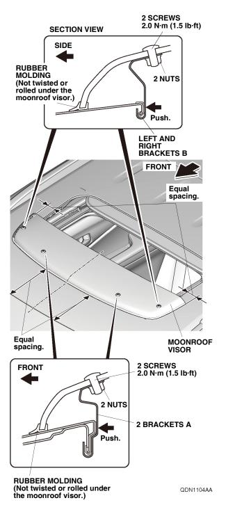
14. Tighten the two screws and two nuts on the front of the vehicle first, then tighten the two screws and two nuts on each side. Tighten while applying pressure so that there is no gap between the roof panel and the brackets A and B. Torque the screws to 2.0 N·m (1.5 lb·ft). 15. Remove the shop towels inserted in step 2. Remove the IMPORTANT INFORMATION label.
