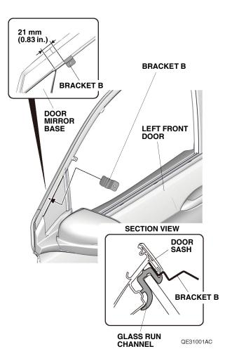
5. Use one alcohol swab to thoroughly clean the area where the left front door visor will attach.
