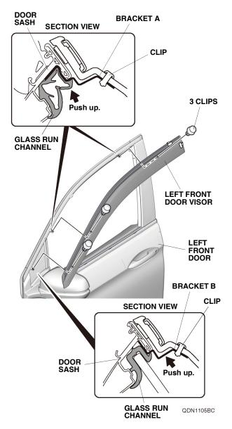
8. Secure the left front door visor to two brackets A and one bracket B with three clips. Make sure to push up on the two brackets A and one bracket B while installing the three clips.
