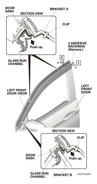
Using a soft towel, press and hold the left front door visor against the door sash for 30 seconds.
