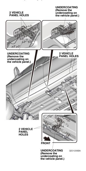
3. Loosely install the left bracket A, left bracket B, and left bracket C to the vehicle panel with six flange bolts.
