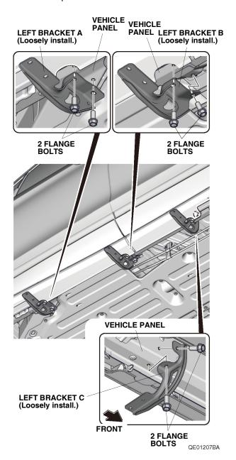
4. With the help of an assistant, install the left running board to the left bracket A, left bracket B, and left bracket C with six flange bolts. Torque the flange bolts to 27 N·m (20 lb·ft).
