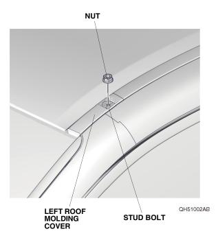
4. Using a plastic trim tool, carefully remove the left roof molding as shown.
