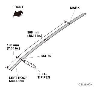
9. While wearing eye protection, use an air saw to cut the left roof molding at the two marks made in step 8. Remove any burrs.
