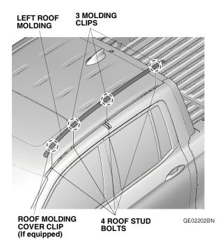
5. Remove the three molding clips from either the left roof molding or the roof stud bolts.
