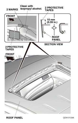
Remove the adhesive backing from the two protective tapes, and attach one to the roof panel at each of the two marks you made. Wrap 10 mm (0.39 in.) of protective tape around the lip of the moonroof opening. 6. Locate the second indentations from the right front corner and left front corner of the moonroof opening. Using isopropyl alcohol on a shop towel, clean the roof panel where the protective tape will attach.
