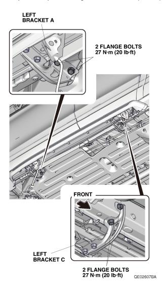
14. Line up the green tape on the left running board harness with the hole on left bracket A and secure the left running board harness to left bracket A with one wire tie.
