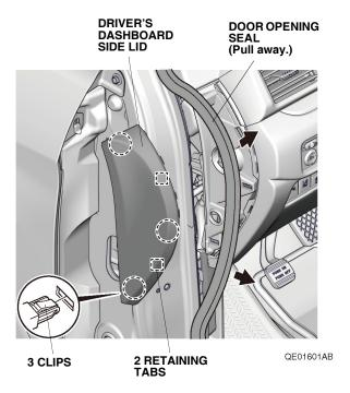
6. Remove the driver's dashboard lower cover, unplug the vehicle connectors, and release the vehicle sensor.
