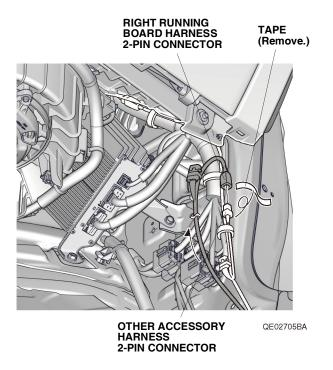
38. Bundle up the excess right running board harness and secure it to the vehicle harness with two wire ties. Go to step 42.
