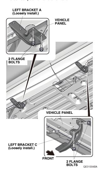
12. With the help of an assistant, install the left running board to the left bracket A and left bracket C with four flange bolts. Torque the flange bolts to 27 N·m (20 lb·ft).
