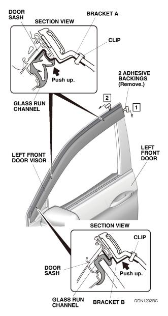
11. Using a soft towel, press and hold the left front door visor against the door sash for 30 seconds.
