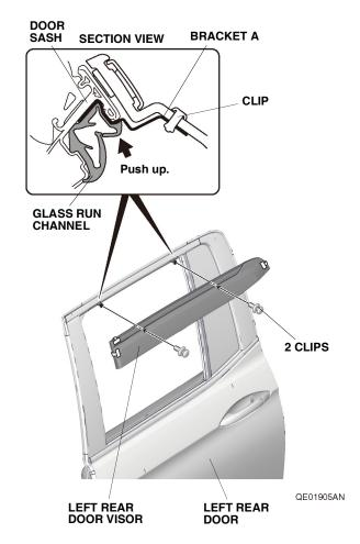
18. Secure the left rear door visor to two brackets A with two clips. Make sure to push up on the two brackets A while installing the two clips.
