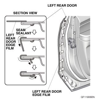
20. Using a shop towel, wipe the 3M protective tape application solution from the left rear door edge film. Allow the left rear door edge film to dry thoroughly.
