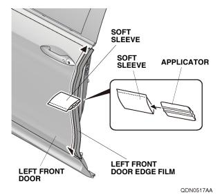
11. Slowly remove the protective film from the left front door edge film.
