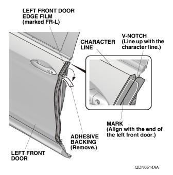
6. Line up the mark on the left front door edge film with the end of the left front door. While applying light pressure, carefully remove the adhesive backing. Go to step 10.
