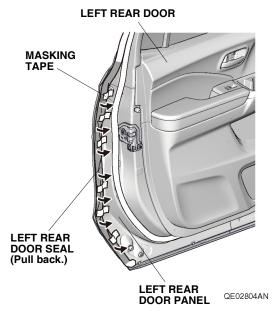
2. Using the alcohol swab, thoroughly clean the area where the left rear door edge film will attach.
