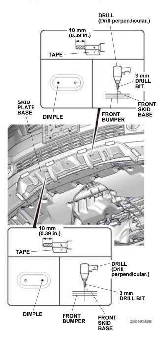
While holding the skid plate base against the front bumper, secure the skid plate base to the front bumper with the two self-tapping screws. Remove the masking tape attached in step 5.
