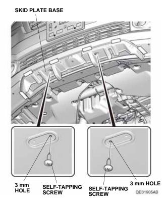
Make sure there are no gaps between the outside 8. edge of the skid plate base and the front bumper. If a gap is found on the outside edge of the skid plate base, remove the self-tapping screws and realign the skid plate base. Repeat steps 5 through 7 to drill in the two alternate locations, then install the selftapping screws in the alternate locations.
