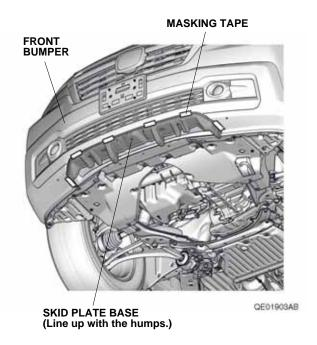
Locate the two dimples on the skid plate base. While
