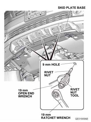
14. Turn the 19 mm ratchet wrench clockwise while holding the rivet nut tool perpendicular to the skid plate base. Turn the nut until firm resistance is felt. Several turns are required.
