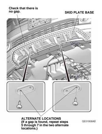
While wearing eye protection, drill the front bumper through each 9 mm hole in the skid plate base with a 9 mm drill bit. Remove any burrs. NOTE: Wrap tape around a 9 mm drill bit 10 mm
