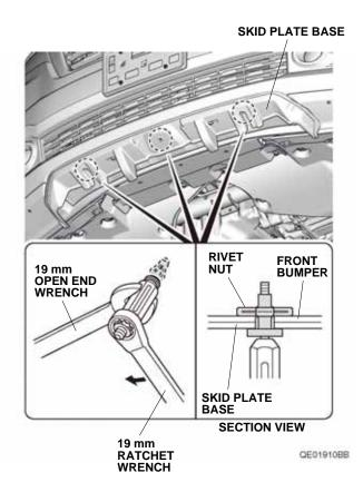
15. Remove the rivet nut tool from the rivet nut by turning the rivet nut tool body counterclockwise.
