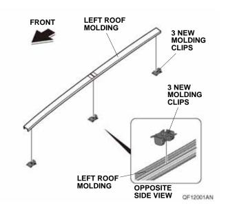
11. Install the left roof molding cover and left roof molding with the three molding clips and one roof molding cover clip. Line up the marks made in step 1 on the vehicle panel and left roof molding.
