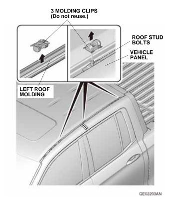
Remove any excess sealant from the four roof stud bolts.
