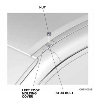
4. Using a plastic trim tool, carefully remove the left roof molding as shown.
