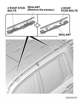
7. Remove the left roof molding cover from the left roof molding as shown.
