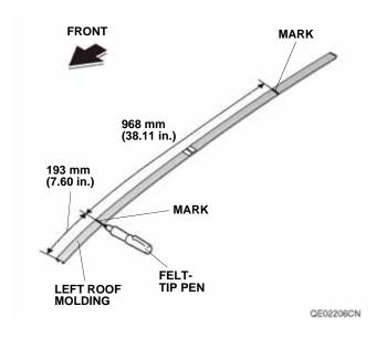
While wearing eye protection, use an air saw to cut the left roof molding at the two marks made in step 8. Remove any burrs.
