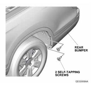
2. Install one spring nut on the left rear splash guard as shown.
