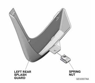
3. Install one spring nut on the left rear inner fender as shown.
