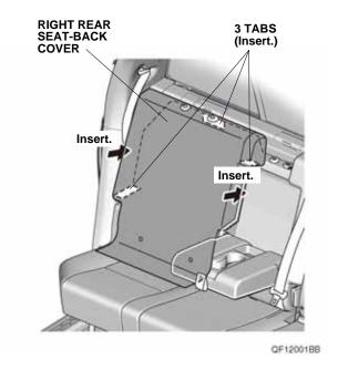
5. Raise the armrest and right rear seat cushion. Pull out the right rear seat-back cover between the right rear seat-back and right rear seat cushion. Insert the right rear seat-back cover between the right rear seat-back and each anchor, then secure the right rear seat-back cover with one fastener.
