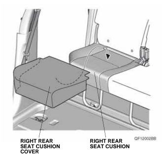
18. Raise the right rear seat cushion and secure the right rear seat cushion cover with the six hooks and two tabs.
