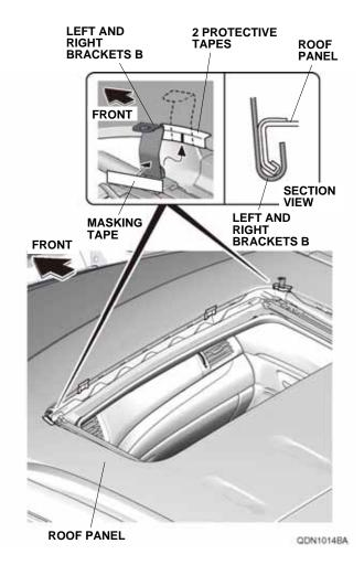
9. Place the two brackets A into position over the two protective tapes and around the lip of the roof panel, and tape them into position with strips of masking tape. Be sure to line up the lower end of the brackets A with the second indentation.
