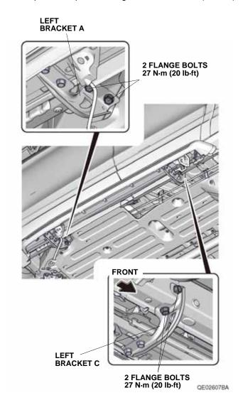
14. Line up the green tape on the left running board harness with the hole on left bracket A and secure the left running board harness to left bracket A with one wire tie.
