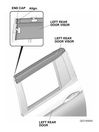
20. While applying light pressure against the left rear door visor, carefully remove the adhesive backings as shown. Make sure to push up on the brackets while removing the adhesive backings.
