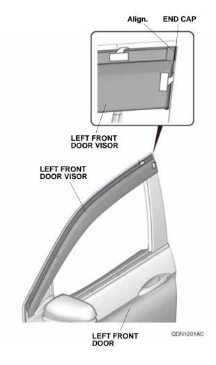
10. While applying light pressure against the left front door visor, carefully remove the adhesive backings in the order shown. Make sure to push up on the brackets while removing the adhesive backings.
