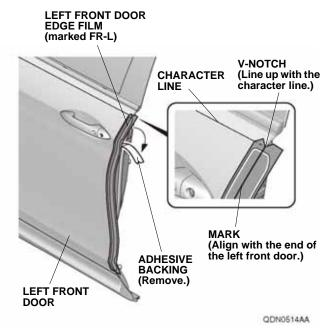
Line up the mark on the left front door edge film with the end of the left front door. While applying light pressure, carefully remove the adhesive backing. Go to step 10.
