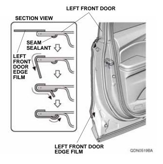
Using a shop towel, wipe the 3M protective tape application solution from the left front door edge film.
