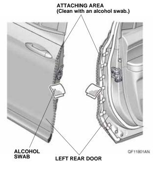
Open the left front door. Using the alcohol swab, thoroughly clean the area where the left front door edge film will attach.
