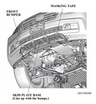
6. Locate the two dimples on the skid plate base. While wearing eye protection, drill the inside dimples on the skid plate base with a 3 mm drill bit. Make sure to drill through the skid plate base and front bumper. Remove any burrs.
