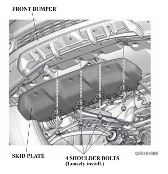
19. Loosely secure the skid plate to the front bumper with one 6 x 24 mm bolt, two 6 x 40 mm bolts, and three washers.
