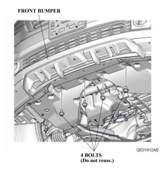
18. Loosely install the skid plate to the front bumper with the four shoulder bolts.
