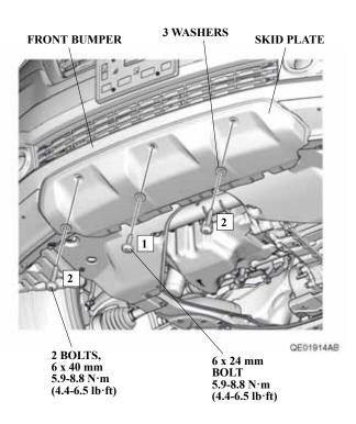
20. Tighten the 6 x 24 mm bolt first, then tighten the two 6 x 40 mm bolts on each side. Tighten while applying pressure so that there is no gap between the skid plate and the skid plate base. Torque the bolts to 5.9-8.8 N·m (4.4-6.5 lb·ft).
