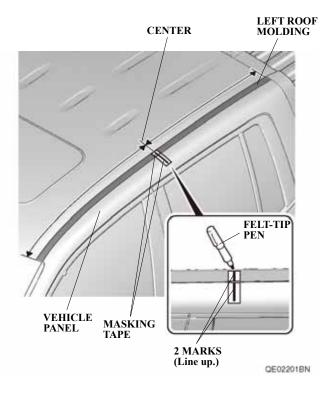
Using a plastic trim tool, carefully remove the left roof molding.
