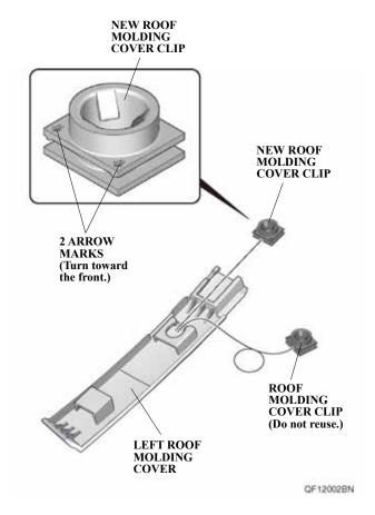
10. Install the left roof molding cover and left roof molding with the three molding clips and one roof molding cover clip. Line up the marks made in step 1 on the vehicle panel and left roof molding.
