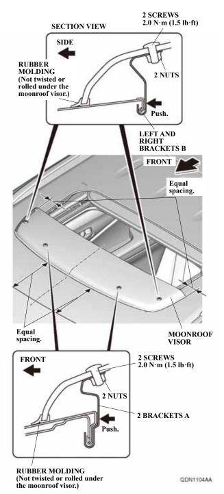
14. Tighten the two screws and two nuts on the front of the vehicle first, then tighten the two screws and two nuts on each side. Tighten while applying pressure so that there is no gap between the roof panel and the brackets A and B. Torque the screws to 2.0 N·m (1.5 lb·ft).
