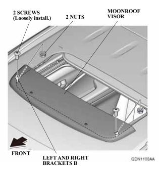
12. Install the brackets against the body as shown.
