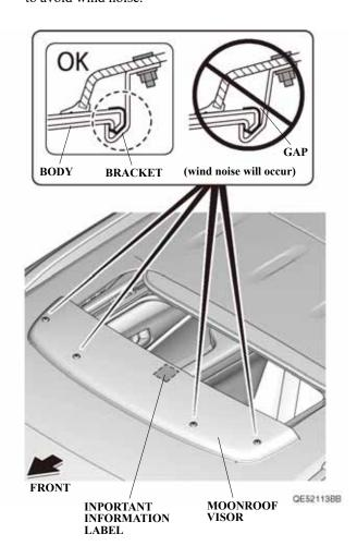
13. Position the moonroof visor with equal spacing on each side. Check that the rubber molding is not twisted or rolled under the moonroof visor.
