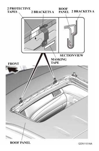
10. Set the moonroof visor on the vehicle roof in front of the moonroof opening, and adjust its position so the holes in the moonroof visor are lined up with the bracket A holes. Loosely install the moonroof visor to the brackets A with two screws and two nuts. Remove the strips of masking tape from the brackets A.
