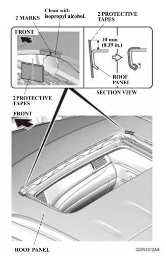
5. Remove the adhesive backing from the two protective tapes, and attach one to the roof panel at each of the two marks you made. Wrap 10 mm (0.39 in.) of protective tape around the lip of the moonroof opening.
