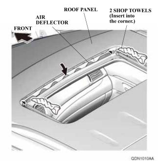
2. Open the moonroof. Roll up two shop towels, and insert them between the roof panel and air deflector to lower the air deflector. Be careful not to damage the air deflector.
