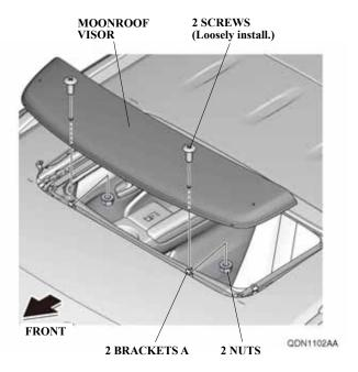
11. Loosely install the moonroof visor to the brackets B with two screws and two nuts. Remove the strips of masking tape from the brackets B.
