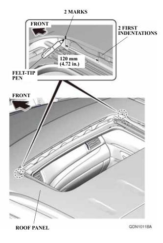
4. Using isopropyl alcohol on a shop towel, clean the roof panel at each of the two marks you have made but do not wipe off the marks.
