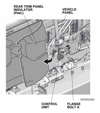
19. Remove the tape to free the vehicle 12-pin connector and plug it to the control unit.
