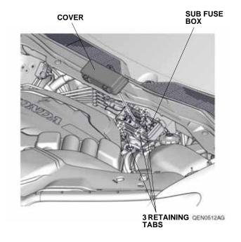
31. Plug the two 7.5 A blade fuses and the two 20 A blade fuses into the sub fuse box.
