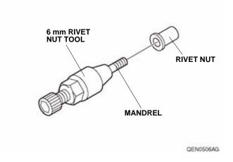
22. Insert the rivet nut into the hole in the trailer hitch and insert the hex wrench in the 6 mm rivet nut tool. NOTE: Rivet nut may be a tight fit into the vehicle hole. If they do not slide in easily, use a hammer to tap them into place.
