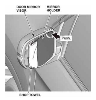
3. Remove the mirror holder, and unplug the vehicle connectors.
