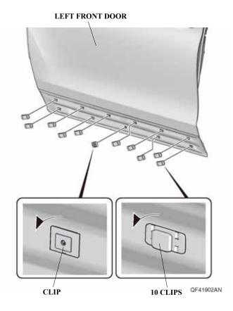
4. Reinstall the 11 clips removed in step 3 and one screw removed in step 1 to the left front door lower trim.
