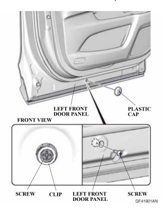
2. Slide and remove the left front door lower trim from the left front door.
