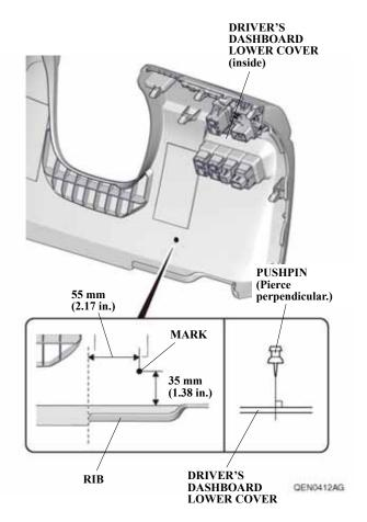
81. While wearing eye protection, drill the pierced mark on the driver's lower cover with a 3 mm drill bit.
