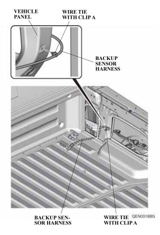
57. Using isopropyl alcohol on a shop towel, thoroughly clean the vehicle panel where the aluminum tape will attach.
