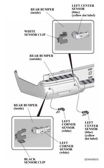
71. Secure the left corner sensor (white) and left center sensor (blue) with white sensor clip and black sensor clip as shown.
