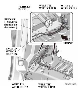
54. Remove the vehicle grommet. Route the backup sensor harness through the vehicle grommet hole. Install the floor carpet.
