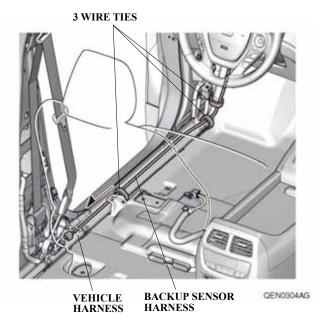
40. Secure the backup sensor harness to the vehicle harness with three wire ties.
