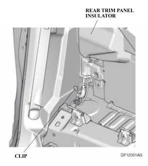
46. Using a utility knife, cut off the rear trim panel insulator as shown.
