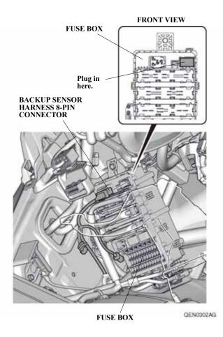
38. Secure the backup sensor harness to the vehicle harness with two wire ties.
