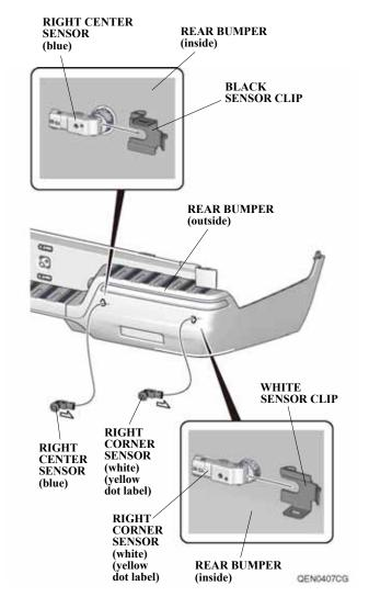
73. Secure the right corner sensor (white) and right center sensor (blue) with white sensor clip and black sensor clip as shown.
