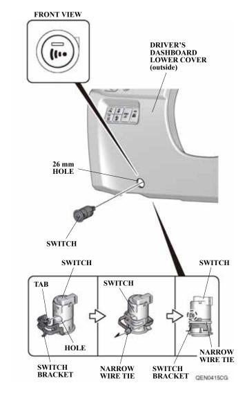
84. Line up the tab on the switch bracket with the hole on the switch and secure the switch bracket to the switch with one narrow wire tie.
