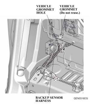
55. Install the backup sensor harness grommet into the vehicle grommet hole.
