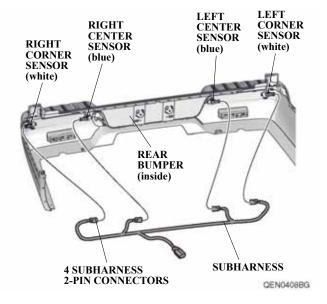
75. Secure the subharness to the four tabs on the rear bumper.
