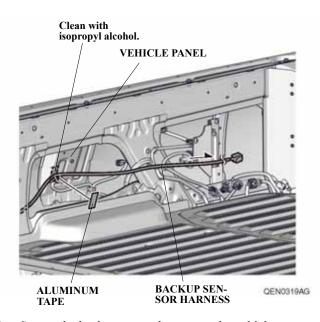
58. Secure the backup sensor harness to the vehicle panel with one aluminum tape as shown.
