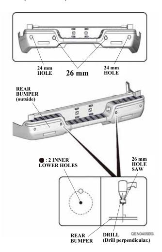
70. Insert the left corner sensor (white) and left center sensor (blue) into the rear bumper.
