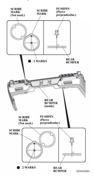
67. While wearing eye protection, drill the eight pierced marks with a 3 mm drill bit from the painted side of the rear bumper.
