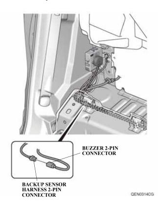
53. Bundle up the excess buzzer harness and secure the buzzer harness and backup sensor harness to the vehicle panel with one wire tie with clip A and one wire tie with clip B.
