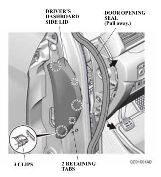
3. Remove the driver's dashboard lower cover release the vehicle sensor.
