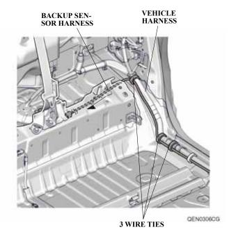
43. Secure the backup sensor harness to the vehicle panel with one wire tie with clip A and two wire ties with clip B.
