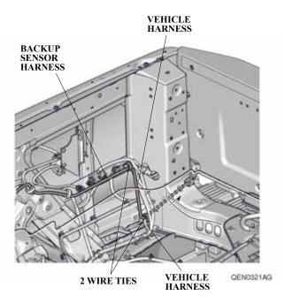
61. Secure the backup sensor harness to the vehicle harness with three wire ties.
