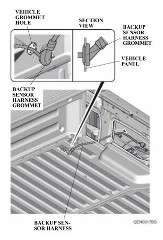
56. Secure the backup sensor harness to the vehicle panel with one wire tie with clip A.
