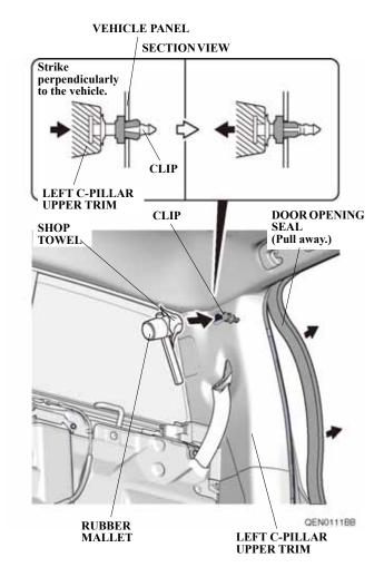
20. Using a rubber mallet wrapped with a shop towel, lightly tap the area marked "SIDE CURTAIN AIRBAG" on the left C-pillar upper trim to push in the clip.
