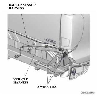
62. Secure the backup sensor harness to the vehicle harness with one wire tie.
