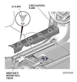
5. Pull away the door opening seal and remove the driver's kick panel.
