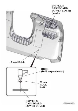
83. Install the switch into the 26 mm hole in the driver's dashboard lower cover.
