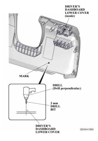
82. While wearing eye protection, enlarge the 3 mm hole to 26 mm using a 26 mm hole saw. Remove any burrs.
