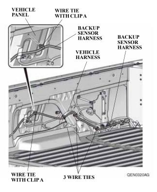
60. Secure the backup sensor harness to the vehicle harness with two wire ties.
