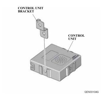
48. Insert the control unit bracket into the hole in the vehicle panel. Secure the control unit bracket and backup sensor harness ground terminal with one ground bolt.
