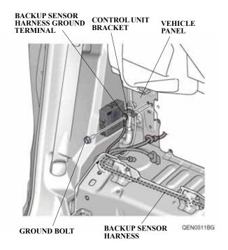
49. Plug the backup sensor harness 14-pin connector into the control unit.
