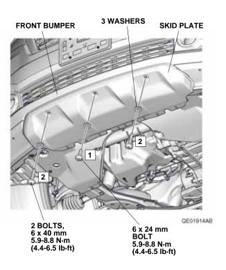
20. Tighten the 6 x 24 mm bolt first, then tighten the two 6 x 40 mm bolts on each side. Tighten while applying pressure so that there is no gap between the skid plate and the skid plate base. Torque the bolts to 5.9-8.8 N·m (4.4-6.5 lb·ft).
