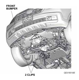
4. Install the left air dam with the two retaining tabs, two washer-bolts, and one clip removed in step 1. Install the right air dam the same way.
