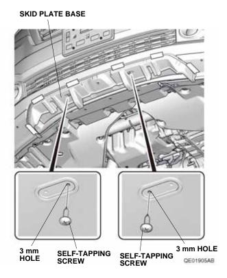
8. Make sure there are no gaps between the outside edge of the skid plate base and the front bumper. If a gap is found on the outside edge of the skid plate base, remove the self-tapping screws and realign the skid plate base. Repeat steps 5 through 7 to drill in the two alternate locations, then install the self-tapping screws in the alternate locations.
