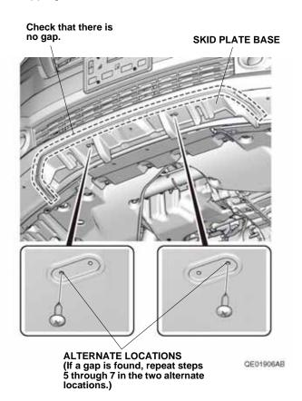
While wearing eye protection, drill the front bumper through each 9 mm hole in the skid plate base with a 9 mm drill bit. Remove any burrs.
