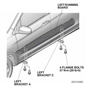
5. Tighten the four flange bolts loosely installed in step 3. Torque the flange bolts to 27 N·m (20 lb·ft).
