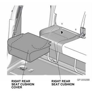
18. Raise the right rear seat cushion and secure the right rear seat cushion cover with the six hooks and two tabs.
