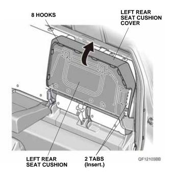
Secure the left rear seat cushion cover with the two fasteners.
