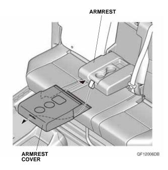
8. Raise the armrest. Pull out the armrest cover between the armrest and the rear seat-back and secure the armrest cover with the fasteners as shown.
