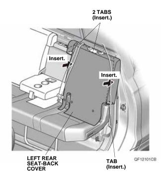
11. Raise the armrest and left rear seat cushion. Pull out the left rear seat-back cover between the left rear seat-back and left rear seat cushion. Insert the left rear seat-back cover between the left rear seat-back and each anchor, then secure the armrest cover and the left rear seat-back cover with the three fasteners.
