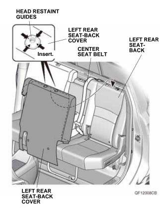
10. Insert the left rear seat-back cover and the three tabs into the left rear seat-back.
