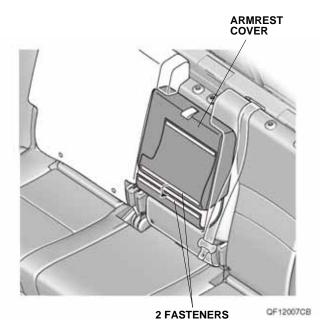
Pull down the armrest. Fit the left rear seat-back cover onto the left rear seat-back through the center seat belt. Insert the left seat-back cover under each head restraint guide.
