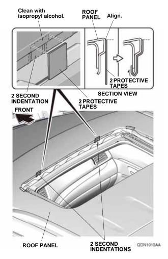
7. Remove the adhesive backing from the two protective tapes, and attach one to the roof panel at each indentation.
