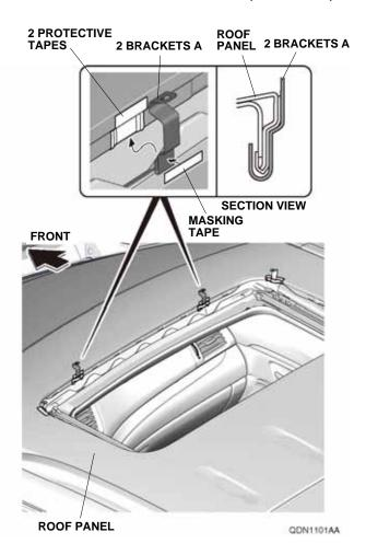
10. Set the moonroof visor on the vehicle roof in front of the moonroof opening, and adjust its position so the holes in the moonroof visor are aligned with the bracket A holes. Loosely install the moonroof visor to the brackets A with two screws and two nuts. Remove the strips of masking tape from the brackets A.
