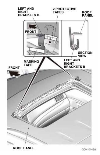
Place the two brackets A into position over the two protective tapes and around the lip of the roof panel, and tape them into position with strips of masking tape. Be sure to align the lower end of the brackets A with the second indentation.
