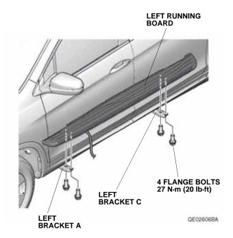
13. Tighten the four flange bolts loosely installed in step 11. Torque the flange bolts to 27 N·m (20 lb·ft).
