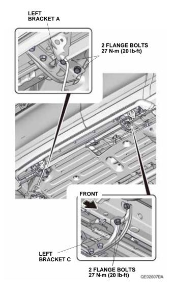
14. Align the green tape on the left running board harness with the hole on left bracket A and secure the left running board harness to left bracket A with one wire tie.
