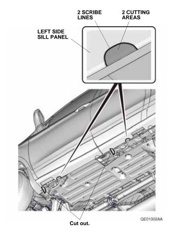
Remove the undercoating as shown. Apply touch-up paint where you removed the undercoating and allow it to dry thoroughly.
