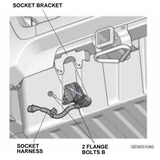
28. Remove the dummy connector from the vehicle 10-pin connector. Plug the socket harness 10-pin connector into the vehicle 10-pin connector.
