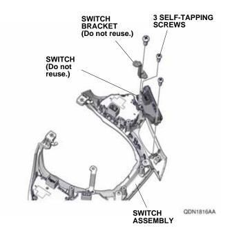
33. Install the new switch bracket and HSW switch on the switch assembly with three self-tapping screws.
