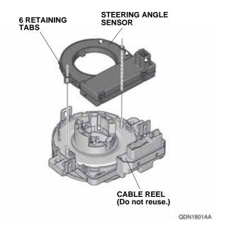
19. Install the steering angle sensor to the new cable reel with six retaining tabs.
