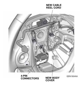
38. Install the two washer-screws and two self-tapping screws.
