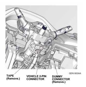
21. Install the new cable reel with three retaining tabs.
