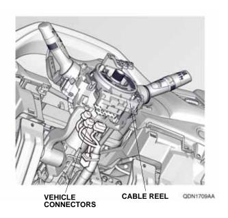
17. To prevent the cable reel from turning, attach masking tape to the cable reel. Remove the cable reel.
