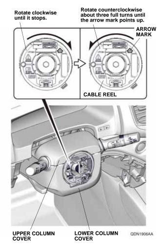
40. Before installing the steering wheel, make sure the front wheels are pointing straight ahead, then center the cable reel. Do this by first rotating the cable reel clockwise until it stops, then rotate it counterclockwise about three full turns. The arrow mark on the cable reel label should point straight up.
