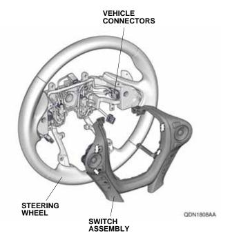
26. If equipped, remove the left and right paddle shifters and unplug the vehicle connectors.
