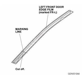
Open the left front door again. Peel back about 50 mm (1.97 in.) of adhesive backing from the left front door edge film. Align the V-notch in the left front door edge film with the character line of the left front door.
