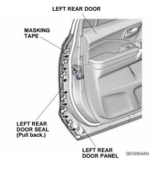
2. Using the alcohol swab, thoroughly clean the area where the left rear door edge film will attach.
