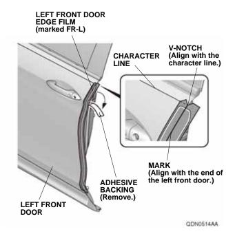
6. Align the mark on the left front door edge film with the end of the left front door. While applying light pressure, carefully remove the adhesive backing. Go to step 10.
