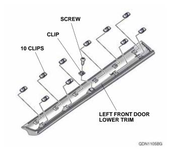
5. Attach masking tape to the left front door lower trim as shown.
