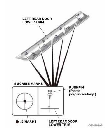
19. While wearing eye protection, drill the five pierced marks to 7 mm. Drill first with a 3 mm drill bit, then finish with a 7 mm drill bit. Remove any burrs. NOTE: Make sure to drill perpendicularly to the left rear door lower trim.
