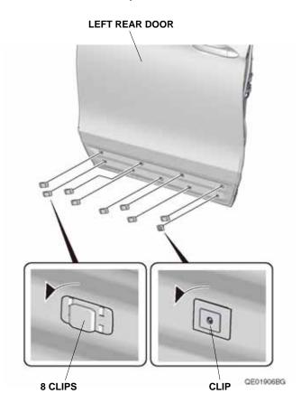
17. Reinstall the nine clips removed in step 16 and one screw removed in step 14 to the left rear door lower trim.
