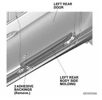
13. Using a rubber roller, apply firm pressure while rolling, especially at the ends, to set the adhesive.
