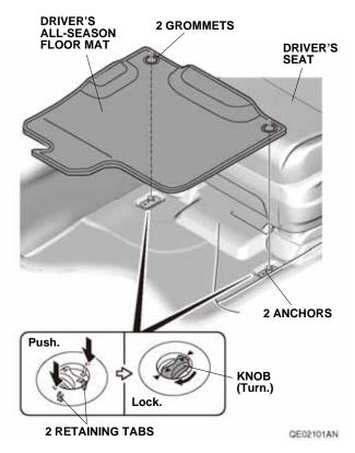
2. Place the grommets in the driver's all-season floor mat over the anchors. Push the grommets into the anchors to secure the retaining tabs, then turn the knobs 90° to secure the driver's all-season floor mat.
