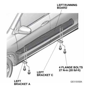
5. Tighten the four flange bolts loosely installed in step 3. Torque the flange bolts to 27 N·m (20 lbf·ft).
