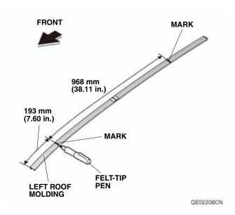
7. While wearing eye protection, use an air saw to cut the left roof molding at the two marks made in step 6. Remove any burrs.
