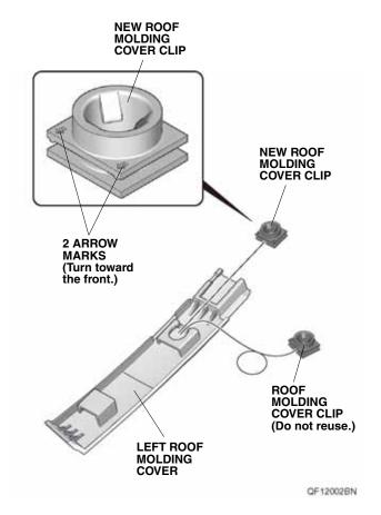
Install the left roof molding cover and left roof molding with the three molding clips and one roof molding cover clip. Align the marks made in step 1 on the vehicle panel and left roof molding.
