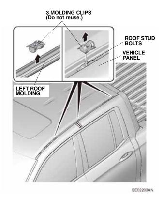
Remove any excess sealant from the four roof stud bolts.
