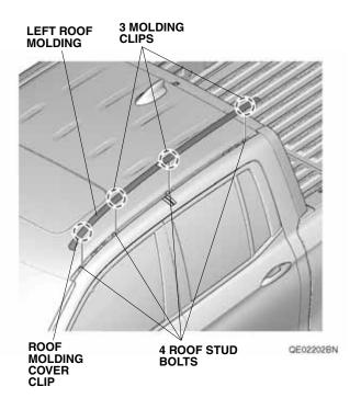
3. Remove the three molding clips from either the left roof molding or the roof stud bolts.
