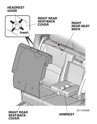
4. Insert the right rear seat-back cover and the three tabs into the right rear seat-back.
