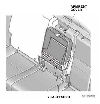
Pull down the armrest. Fit the left rear seat-back cover onto the left rear seat-back through the center seat belt. Insert the left seat-back cover under each headrest guide.
