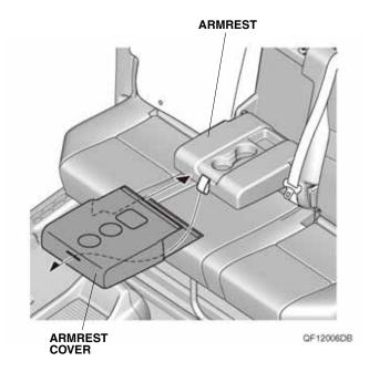
Raise the armrest. Pull out the armrest cover between the armrest and the rear seat-back and secure the armrest cover with the fasteners as shown.
