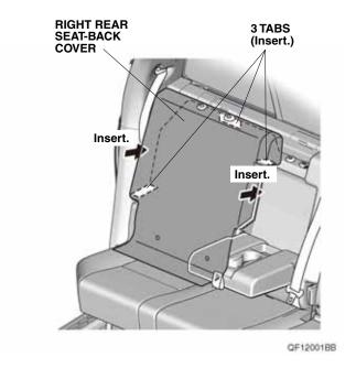
5. Raise the armrest and right rear seat cushion. Pull out the right rear seat-back cover between the right rear seat-back and right rear seat cushion. Insert the right rear seat-back cover between the right rear seat-back and each anchor, then secure the right rear seat-back cover with one fastener.
