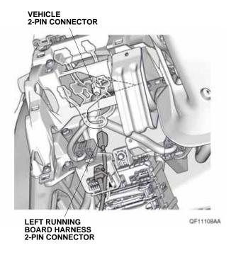
28. Secure the left running board harness to the vehicle harness with two wire ties.
