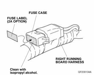
If the vehicle is equipped with the other accessory harness, continue with step 37; otherwise, go to step 39.
