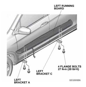
13. Tighten the four flange bolts loosely installed in step 11. Torque the flange bolts to 27 N·m (20 lbf·ft).
