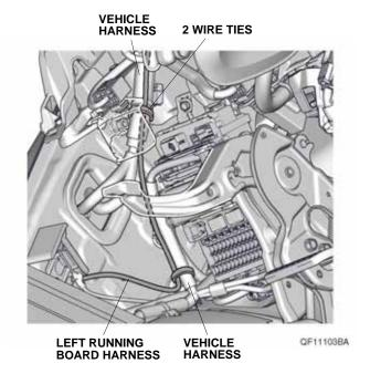
Secure the left running board harness to the vehicle harness with two wire ties.
