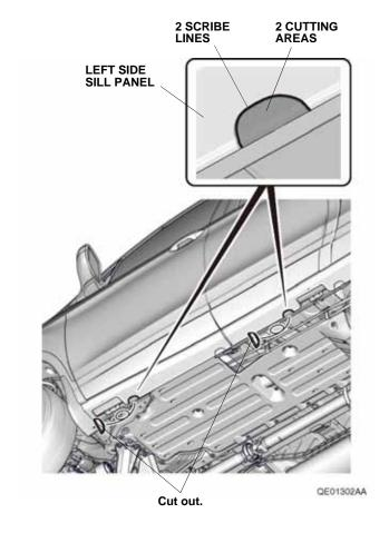
Remove the undercoating as shown. Apply touch-up paint where you removed the undercoating and allow it to dry thoroughly.
