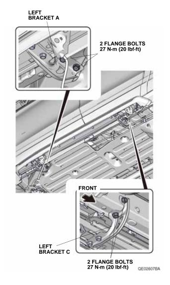
14. Align the green tape on the left running board harness with the hole on left bracket A and secure the left running board harness to left bracket A with one wire tie.
