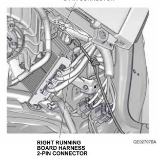
40. Secure the right running board harness to the vehicle harness with two wire ties.
