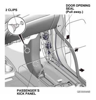
5. Pull away the door opening seal and remove the driver's dashboard side lid.
