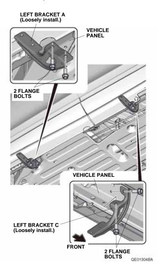
12. With the help of an assistant, install the left running board to the left bracket A and left bracket C with four flange bolts. Torque the flange bolts to 27 N·m (20 lbf·ft).
