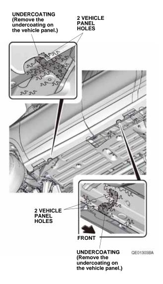
Loosely install left bracket A and left bracket C to the vehicle panel with the four flange bolts.
