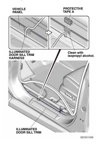
15. Install the protective clip to the protective tape A on the vehicle panel.
