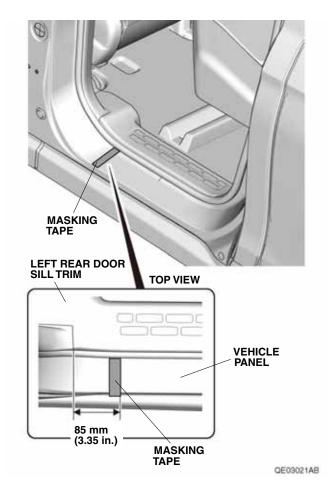
42. Using an alcohol swab, thoroughly clean the vehicle panel where the door sill trim will attach.
