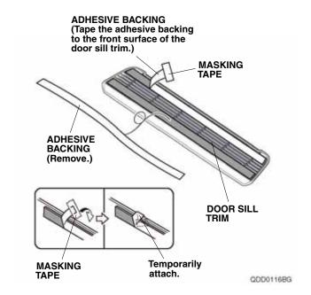
44. Align the door sill trim with the masking tape and install the door sill trim to the vehicle panel.
