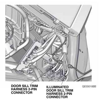
39. Secure the door sill trim harness to the vehicle harness with three wire ties.
