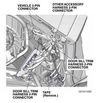
36. Remove the tape from the door sill trim harness and plug the remaining other accessory harness 2-pin connector into the door sill trim harness 2-pin connector. Go to step 38.
