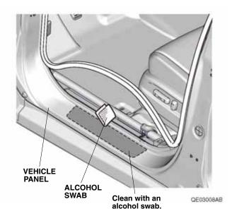
12. Remove the two adhesive backings from the illuminated door sill trim.
