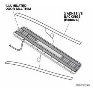
13. Align the cutout shape on the illuminated door sill trim with the bump shape on the vehicle panel. Press firmly on the adhesive part of the illuminated door sill trim.
