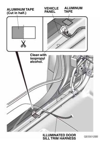
20. Using scissors, cut the aluminum tape in half. Secure the illuminated door sill trim harness to the vehicle panel with one half of the aluminum tape.
