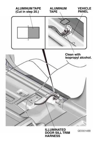
Secure the illuminated door sill trim harness to the vehicle panel with one piece of aluminum tape cut in step 20.
