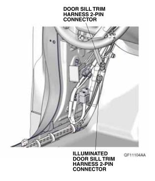
Bundle up the excess door sill trim harness and secure it and the 2-pin connectors to the vehicle harness with three wire ties.
