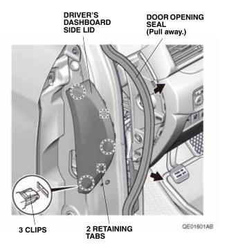
Remove the driver's dashboard lower cover, unplug the vehicle connectors, and release the vehicle sensor.
