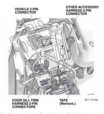
25. Remove the tape from the door sill trim harness and plug the remaining other accessory harness 2-pin connector into the door sill trim harness 2-pin connector. Go to step 27. Without other accessory harness
