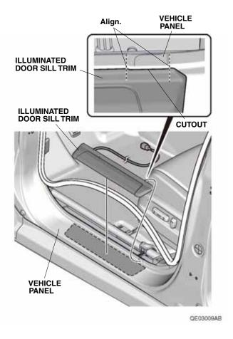
14. Using isopropyl alcohol on a shop towel, thoroughly clean the vehicle panel where the protective tape will attach. Attach one piece of protective tape A to the vehicle panel as shown.
