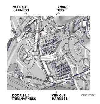
28. Plug the door sill trim harness 2-pin connector into the illuminated door sill trim harness 2-pin connector.
