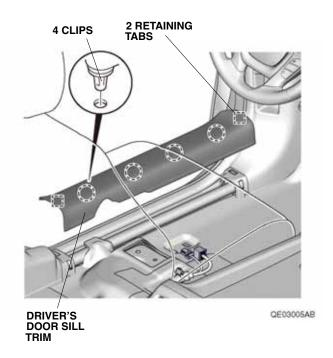
8. Pull away the door opening seal and remove the driver's kick panel.
