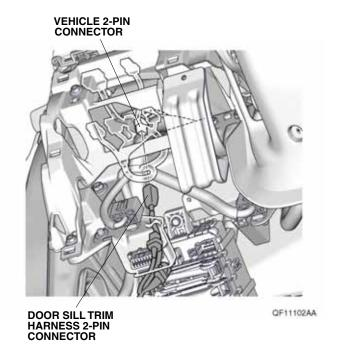
Secure the door sill trim harness to the vehicle harness with two wire ties.
